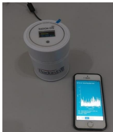
Figure 2: Data collection of Radon Eye RD200 with an iPhone.
